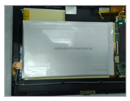
Remove the battery first. Steps for this process be found here <u>Battery</u> <u>Removal</u>
