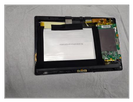
Start by turning the tablet over with the screen down. Carefully use a plastic opening tool to pry the cover off. Start from the corner opposite the hibernate button.
