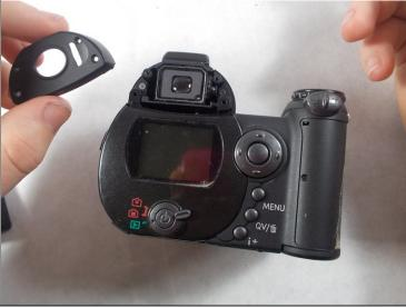
• Use a screwdriver to remove the four viewfinder cover screws.
