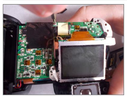
Remove the single screw that connects the circuit board to the motherboard.
