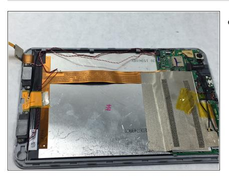
The battery should be removed from the tablet. Now replace the battery.
