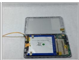
Use a plastic opening tool to free the orange connector ribbon by placing the tool on the connector.
