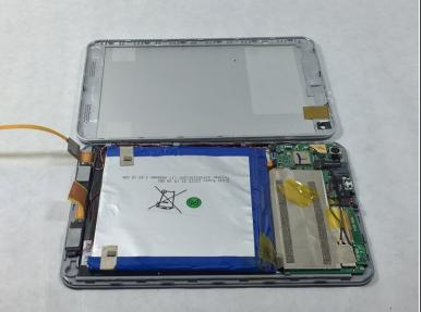
Peel back the three pieces of tape circled in the picture.
