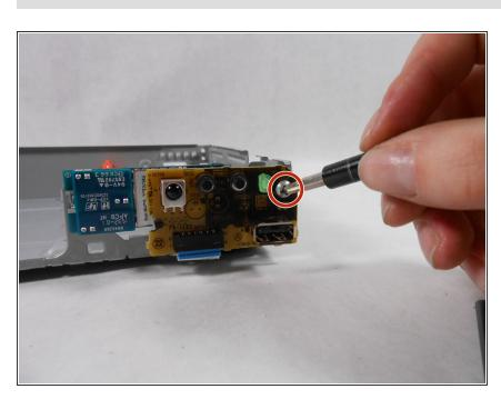
Unscrew the one 5mm Phillips head screw from the front of the device board.
