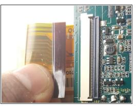
• Lift up the zero insertion force clip with a plastic opening tool and pull out the ribbon cable.
