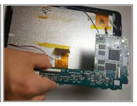
Remove the five 5.7mm PH00 screws with a screwdriver and pull out the motherboard.
