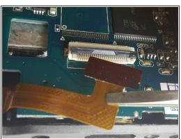
• Lift up the zero insertion force clip with a tweezer and pull out the ribbon cable.
