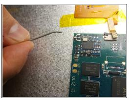
Desolder the grey wire and pull it off the motherboard.
