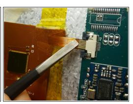
Push out the ribbon cable connectors with a tweezer and pull out the ribbon cable.
