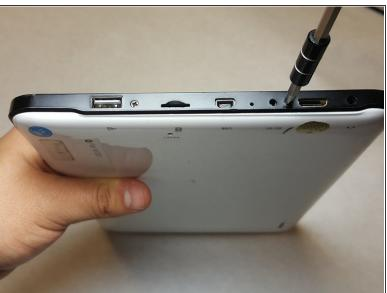
Remove the two 4.1 mm PH1 screws with a Philips screwdriver.
