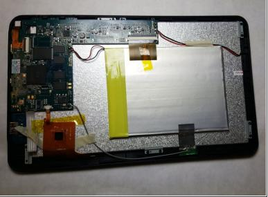
Press the small suction cup on the back cover, and then pull the small suction cup to remove the back cover.
