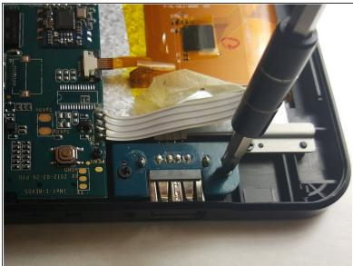
Remove the two 3.8 mm PH1 screw with a Philips screwdriver.
