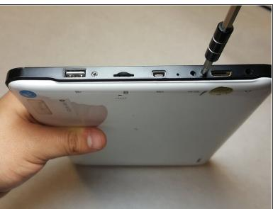
Remove the two 4.1 mm PH1 screws with a Philips screwdriver.
