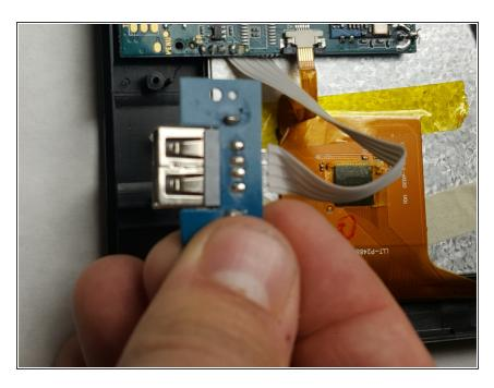
Remove the USB port from it's plastic housing.
