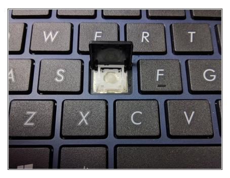
Lift the key and remove from the housing.
