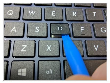
Gently pry the bottom edge of key with a plastic opening tool until it flips up.
