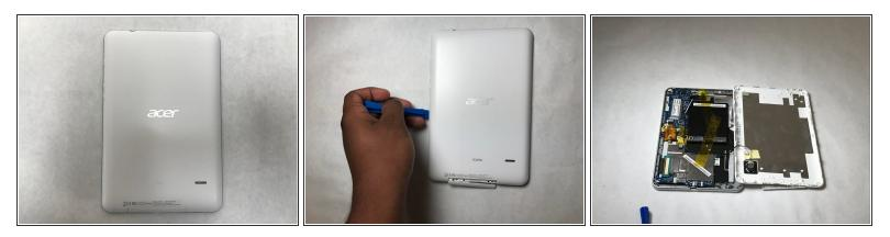
• Open the back cover by prying the casing off with an opening tool.
