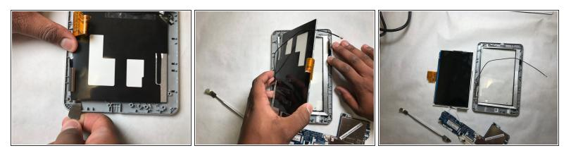
• Peel the LCD display.
