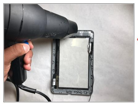
Use a blow dryer to melt the glue between the metal frame and the screen.
