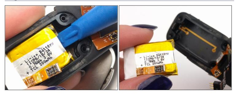
• Pry out the battery using the plastic opening tool.
