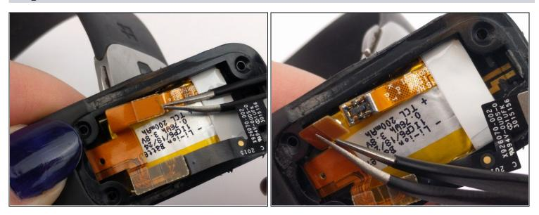
• Detach the orange press-fit (or "pop") connector by using the tweezers.
