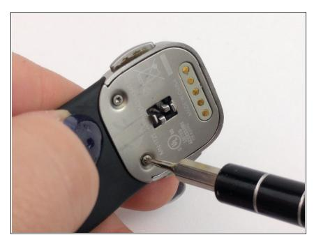
Use the T3 screwdriver to remove the two 2mm screws in the device.
