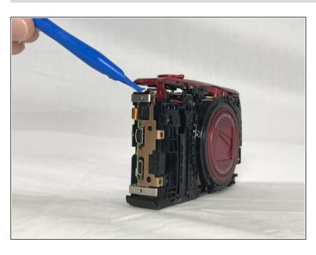
Use an opening tool to gently remove the power and shutter button assembly from the frame.
