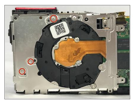
Use a #000 Phillips screwdriver to remove the three 4mm screws that hold the assembly to the frame.
