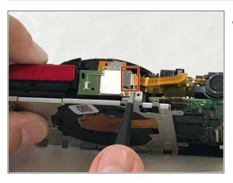
Unplug the assembly from the main no-fuss connector.
