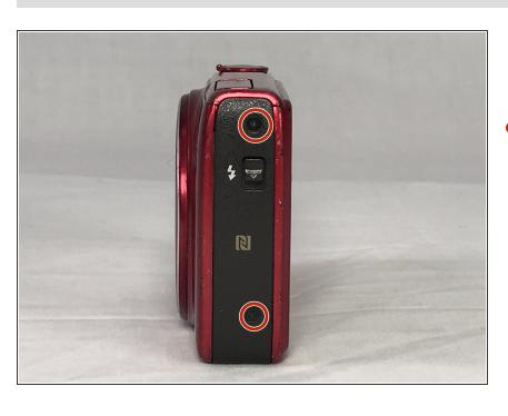
Use a #000 Phillips screwdriver to unscrew the four 4mm screws located on the sides of the camera (2 for each side).
