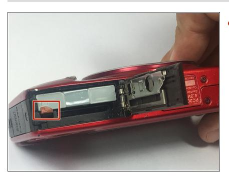
Depress the orange lever holding the battery in place to unlock it.
