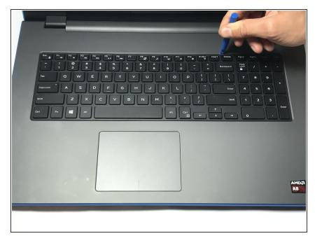
Use a plastic opening tool to gently release the tabs that secure the keyboard to the laptop.
