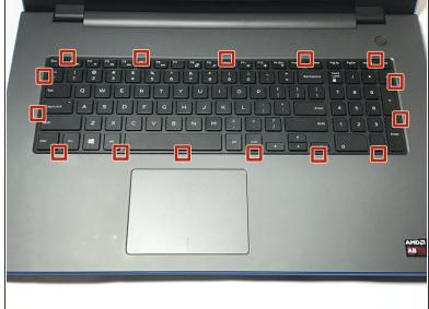
Open the display of the laptop as far as possible, and locate the tabs which secure the keyboard to the laptop.
