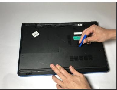
Locate the tabs that hold the base cover to the laptop and use a plastic opening tool to gently release the base cover.
