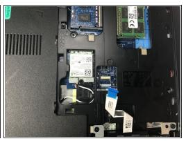
• Disconnect the hard drive ribbon cable from the laptop by lifting the latch which secures it.
