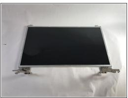
Using a Phillips 0 screwdriver, remove the 10 screws (M2.5 x 4.5) that secure the display panel to the display back-cover.
