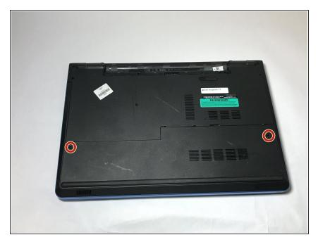
Use a Phillips #0 screwdriver to unscrew the two 8mm screws which secure the base cover.
