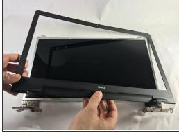
Using the tip of your fingers, gently pry off the display bezel from the back-cover
