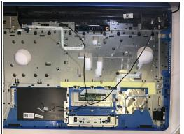
Carefully detach the antenna cables from their respective routing guides
