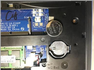
Use a plastic opening tool to gently pry the CMOS battery found at the bottom right of the laptop out of the socket.
