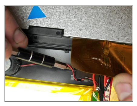
• Carefully remove the speaker cables from the retaining tabs using a thin metal spudger.
