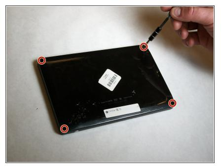
• Use a number 0 screw driver to remove the four screws.
