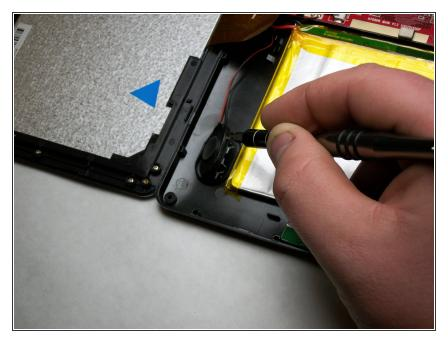
• Pry the speaker out of its molding using a thin metal spudger
