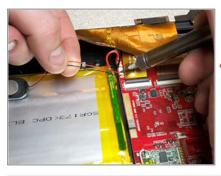
Desolder the two speaker wires from the motherboard using a soldering iron.
