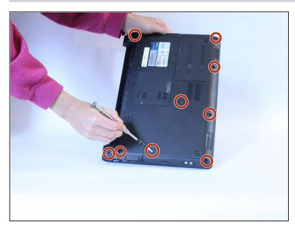
• Once the keyboard is removed, take out the nine 6 mm screws on the back side of the laptop.
