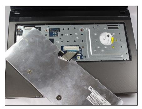
Remove piece of tape that covers the connection between the data cable and the connector.
