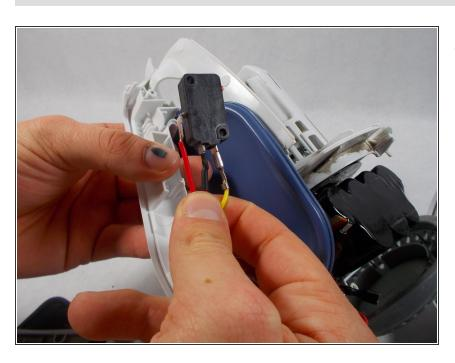
Remove the switch assembly from inside the grey handle.
