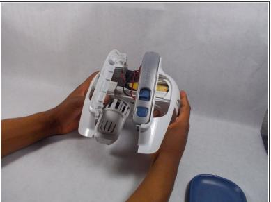
Separate the two halves of the outer shell by pulling them apart.
