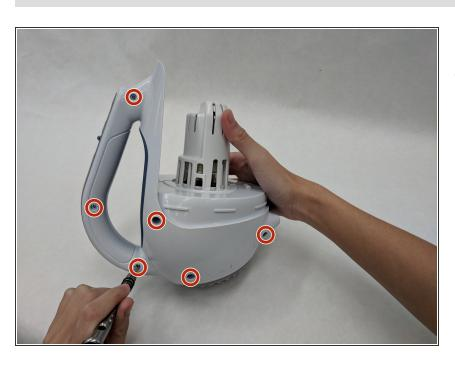
Remove the six exterior 2 mm
