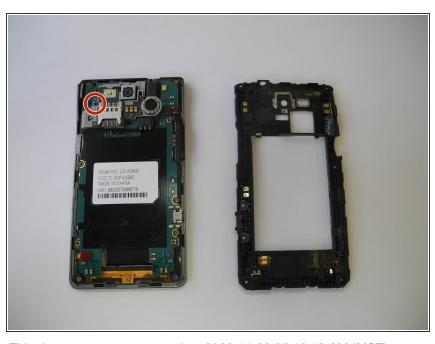
Remove the single Phillip's head screw holding the sim card assembly in place.
