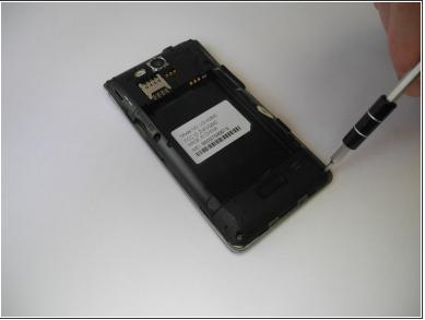
Begin by removing the seven Phillip's head screws on the back of the phone.
