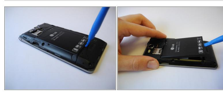
Using the notch located near the bottom center, remove the battery with a prying tool or your fingernail.
