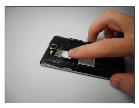
Using your finger, carefully remove the SIM card from its slot by moving it toward the battery area.
