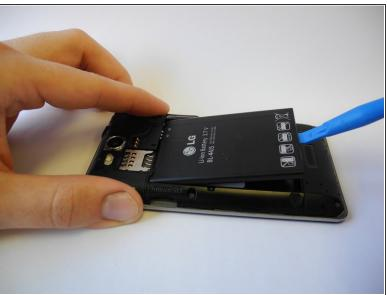
Using the notch located near the bottom center, remove the battery with a prying tool or your fingernail.
