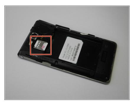
After you have cleaned the battery area, locate the SIM card slot.
