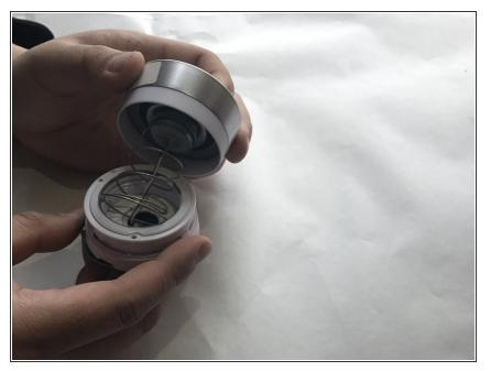
• Pry the spring from the speaker housing using the blue plastic pry tool.
