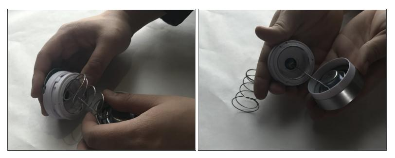
• Unwind the old spring from the wires.
