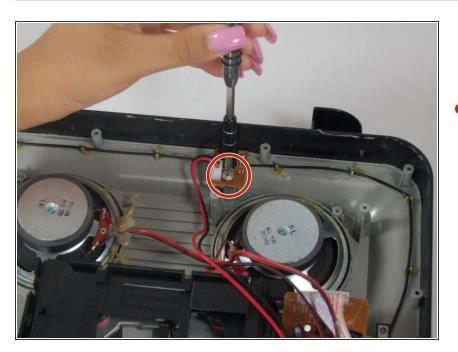
Remove the one (13.5mm in length) srew holding the power connector and cord in place.
