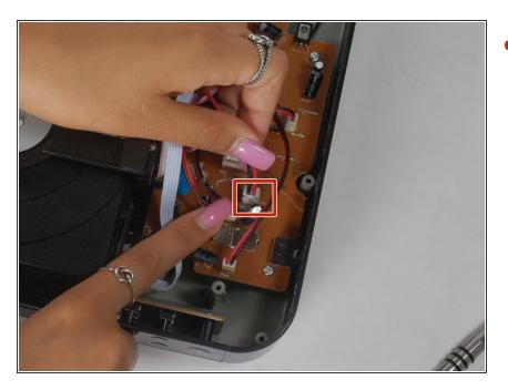
Remove the power cord connected to the motherboard.
