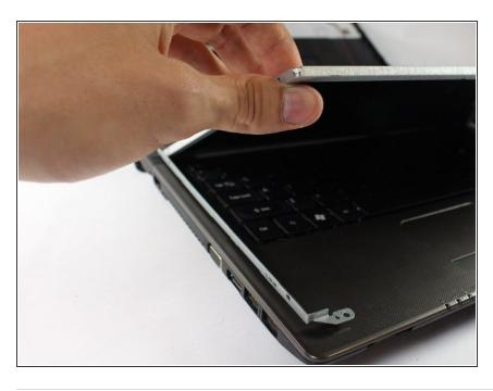
• The screen can be easily removed from its frame now.
