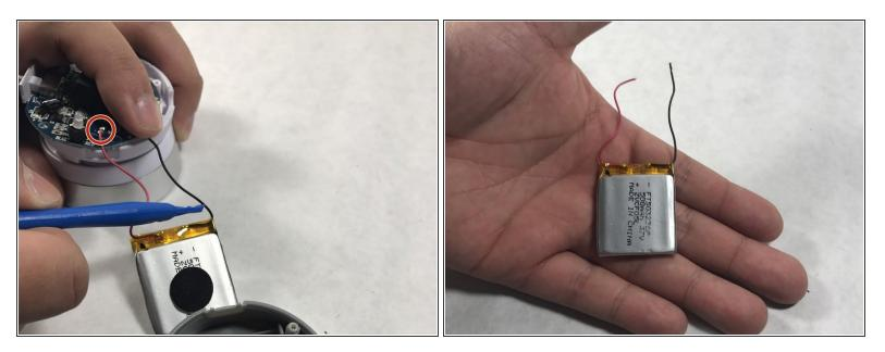
Unsolder the batterie's wires from the circuit board to remove the old battery.
