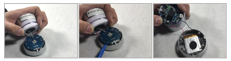
Locate the battery underneath the circuit board.
