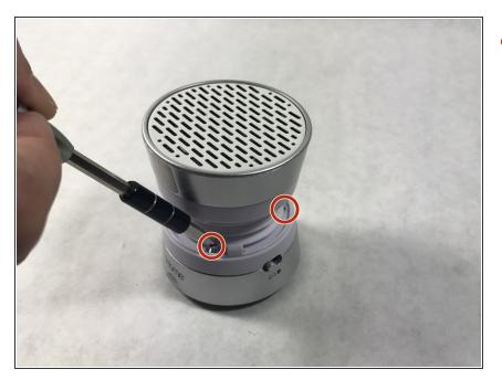
Use a #000 Phillips screwdriver to remove the four 1 mm screws from the bottom half of the speaker.
