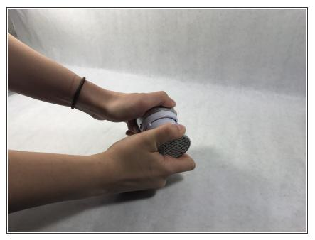
• Push down and turn the top of the speaker clockwise. This will release the clips and expand the speaker.
