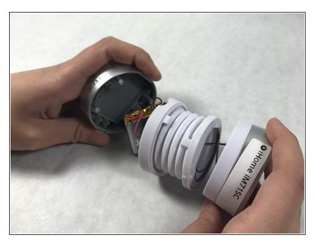
• Remove the now unfastened coverings to expose the internals of the speaker.
