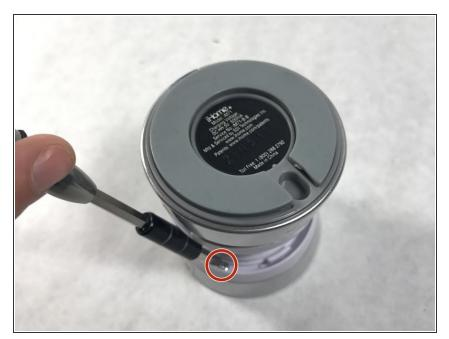
Flip the speaker over and use a #000 Phillips screwdriver to remove three 1mm screws. Unscrew these to unfasten the top.
