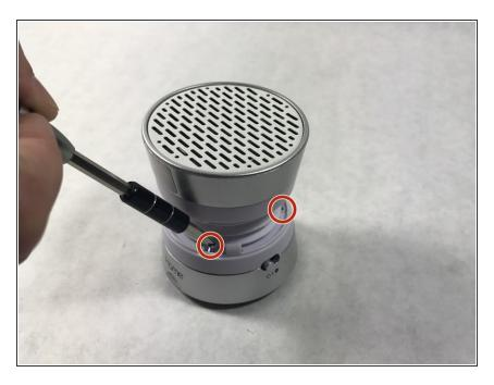
Use a #000 Phillips screwdriver to remove the four 1 mm screws from the bottom half of the speaker.
