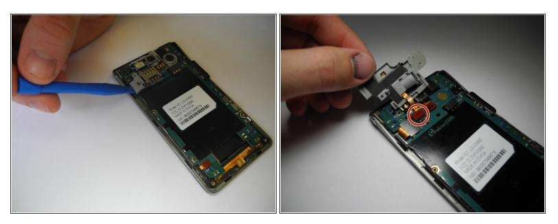
Remove SIM card holding by prying it with opening tool. As you are lifting it, disconnect the ribbon that is connecting the sim card holding and the rest of the phone.
