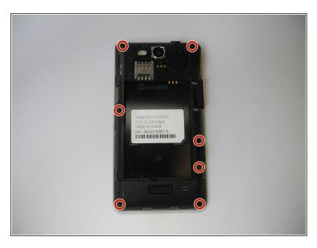
Remove the 7 ph000 screws found on the back of the phone.
