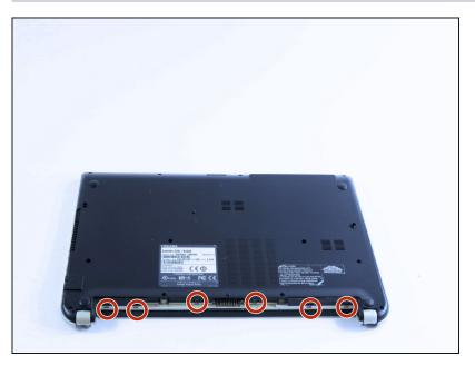
Use a spudger to depress the six white clips connecting the plastic cover
