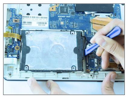
Use an opening tool or your fingers to lift the hard drive out of the laptop.
