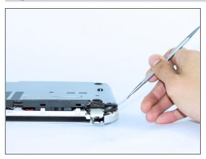
Run the spudger or a <u>plastic</u> <u>card</u> around the entire laptop to release the rest of the clips.
