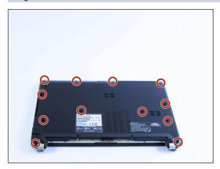
Remove the following twelve 4mm screws with a Phillips #0 screwdriver.
