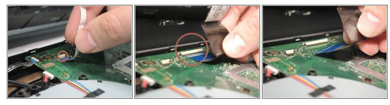
Disconnect these cables by unlocking the ZIF connectors with a spudger.
