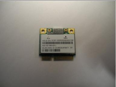
Remove the wireless card along its angle, and insert your replacement card at the same angle.
