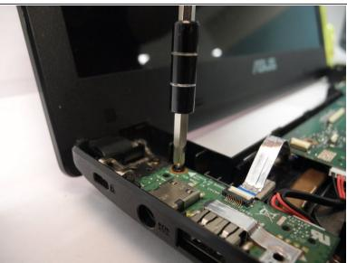
Using a Phillips Head 1 Screwdriver, remove all screws securing the motherboard to the frame of the laptop
