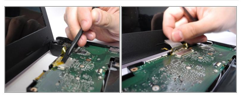
Peel back the tape securing the cable for the laptop's screen. It is not recommended you
