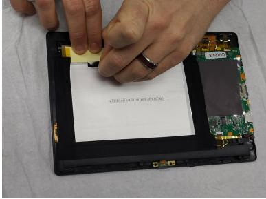
Pick up the magnets from the bottom edge of the tablet next to the keyboard connection and put them in a place that they will not get lost. Then carefully remove all 4 strips of electrical tape.
