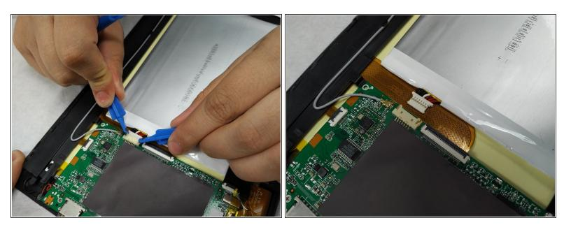
Using a small plastic opening tool; genteelly pull the connection off of the motherboard.
