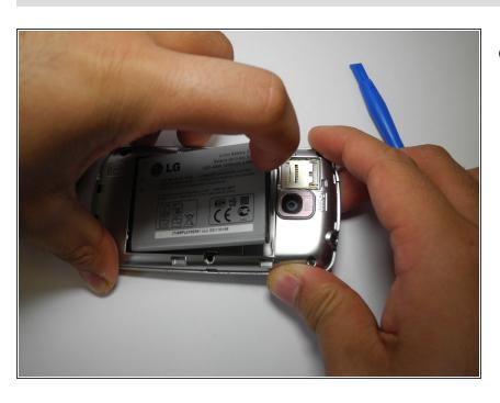
Remove the battery. There's an indentation to the left of the camera lens.
