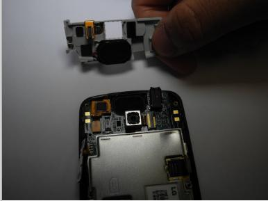
Remove SD card mount. Use a plastic opening tool to assist removal.
