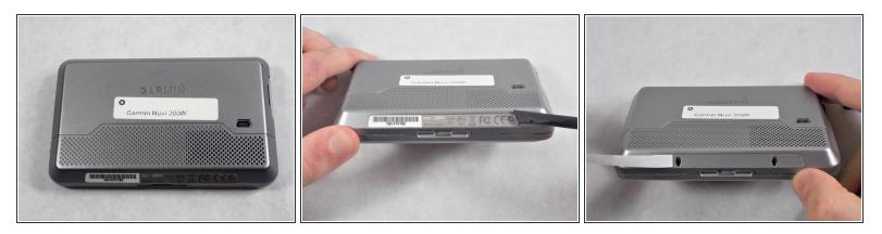
• Peel off the sticker in order to find the two Torx T5 screws.
