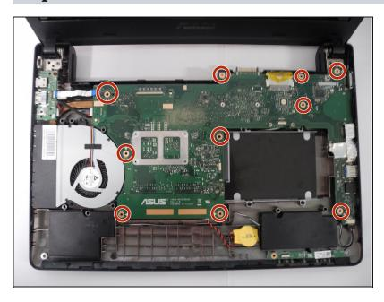
Unscrew the ten 3mm screws with a Phillips Head #1 screwdriver,
