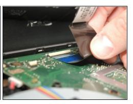
• Use a spudger to lift ZIF tabs up to disconnect the black and the white ribbon cable.
