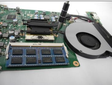
• Unscrew the four screws with a Phillips Head #1 screwdriver to disconnect the fan from the processor.
