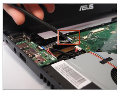
Use a spudger to lift the ZIF connector up to release the ribbon cable.
