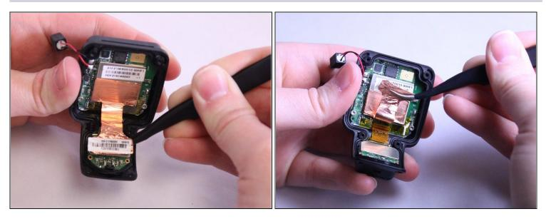
Now lift the smaller square of copper off the front panel. Use the precision <u>tweezers</u> and slide it under the smaller square of copper lining then gently lift it up.
