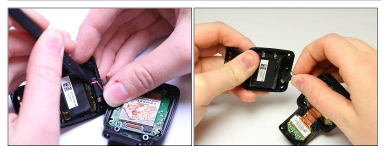
• Gently wiggle the black box vibrator component away from the back panel with your fingers or a Spudger tool.
