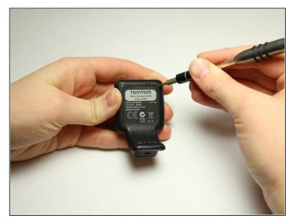
• Flip over the watch and remove the four 3.0 mm Torx head screws with a T4 Torx head screwdriver.
