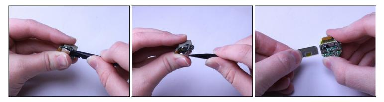
• Get the GPS/Button Component by itself and use the Spudger tool to lift the silver cover off the GPS Component. This will expose the GPS Component.
