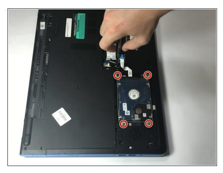
Use a Phillips #0 screwdriver to remove the four 8mm screws which secure the hard drive assembly to the laptop.
