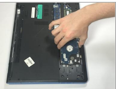
Carefully remove the hard drive and its assembly from the laptop.
