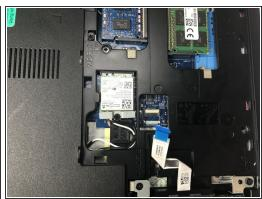
• Disconnect the hard drive ribbon cable from the laptop by lifting the latch which secures it.
