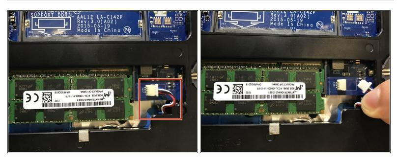
Turn over the laptop, and safely disconnect the speaker cable.
