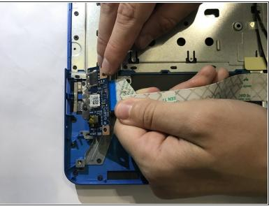
Use a Phillips #0 screwdriver to remove the 5mm screw that secures the I/O board to the palm-rest assembly.
