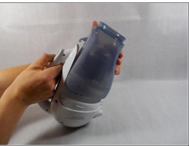
Remove the dustbin by pressing the blue button on the vacuum's handle and lift the bin from the vacuum.
