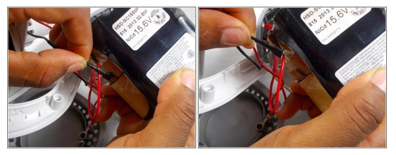
Disconnect the red wire from the battery pack (pull do not twist!) and do the same with the black wire To reassemble your device, follow these instructions in reverse order.
