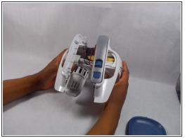
Gently separate the two halves by pulling them apart, revealing the 14 cell battery pack behind the motor.
