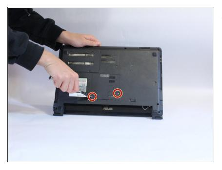
Unscrew the back plate in the middle of the laptop by removing the two 5 mm screws - this will expose the RAM cards.
