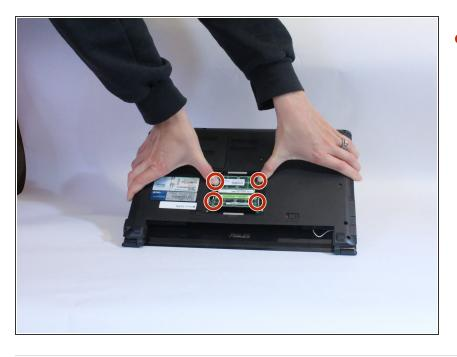
Pull the tabs and then slide the card to remove the RAM cards. To reinsert a new RAM card, slide the card in and then make sure it clips in with the tabs.
