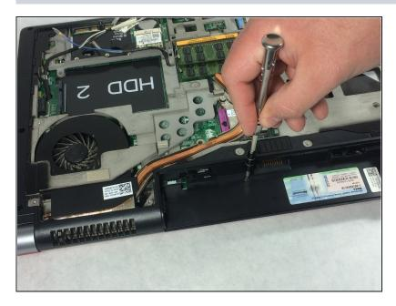
Remove the 4mm ph1 screw under the battery
