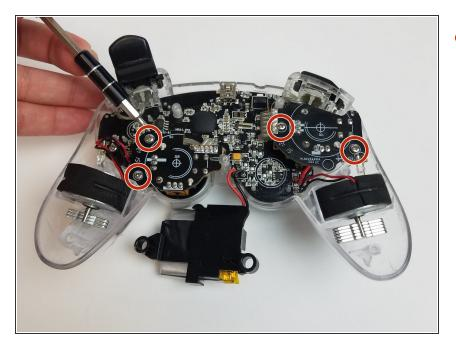
Unscrew the four 9mm Phillips #0 screws that are attached to both joy stick control mini-motherboards. There are two screws for each minimotherboard.
