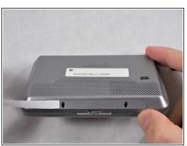
Peel off the sticker in order to find the two Torx T5 screws.
