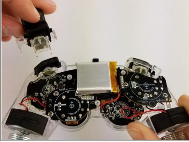
With one hand, hold the controller down and with the other pull up on the lower clear plastic trigger housing to remove it.
