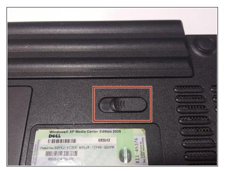
• Locate the slide lock for the battery.
