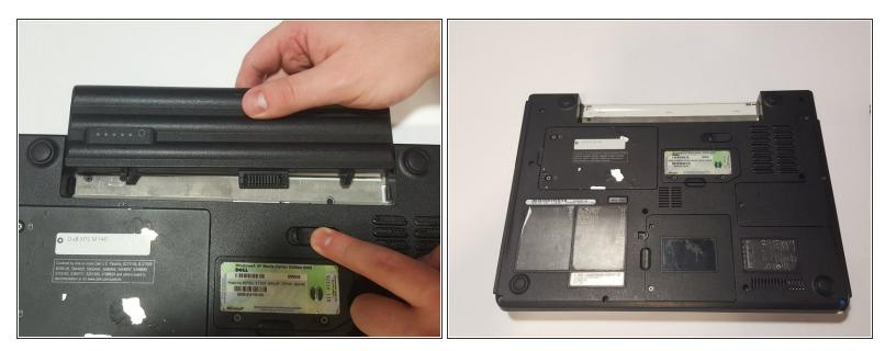
• Slide the lock and pull out the battery.
