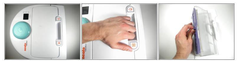
Carefully grasp the back latch and open to reveal filter compartment.
