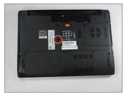
Remove the 7.0 mm screw, circled in the picture, using a Phillips head screwdriver.
