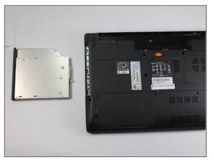
• Remove the drive completely.
