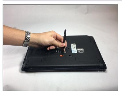
• Use <u>tweezers</u> (or a similar tool) to slide the orange push pin. To release the battery, push it to the left.
