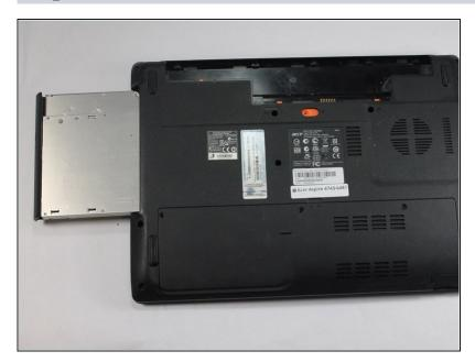
Once the screw is removed, the DVD drive should easily slide out
