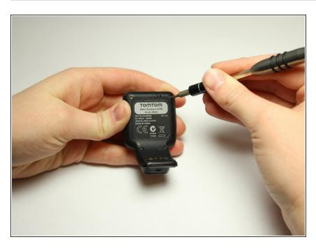
Flip over the watch and remove the four 3.0 mm Torx head screws with a T4 Torx head screwdriver.
