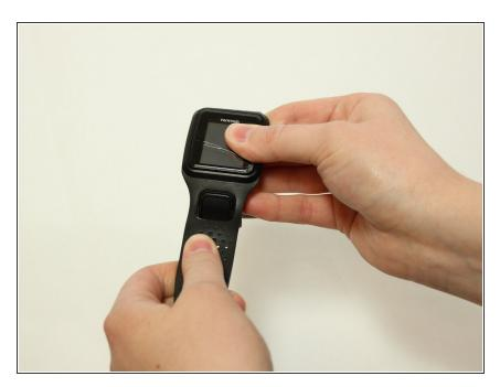
First, lift the bottom part of the band to start removing the wristband from the button area of the watch.
