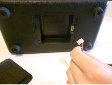
Carefully disconnect the battery cord from its socket. Carefully pinch the ends of the rectangular battery cord connector that is connected to the machine and gently pull the rectangular portion away from the machine so that it disconnects.
