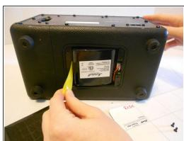
Pull the yellow tab to remove the battery from the amp.
