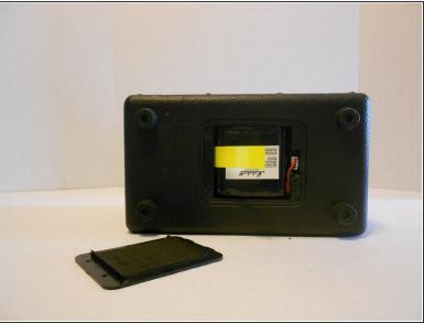
To reassemble, plug in the new battery cord, and insert the battery pack; have the yellow tab repositioned as in step 3.
