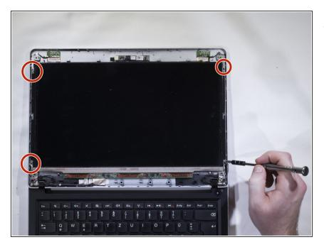
Under the bezel, there are 4, 3mm long M2 screws holding the screen to the hinge. Remove the screws.
