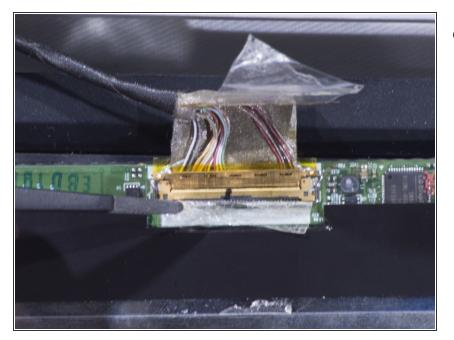
• Underneath the tape there is an exposed connection. The connection cable that plugs into the screen has a securing wire lock that locks the connection in place. The locking wire has a piece of tape that secures it in place to the back of the screen. With the tweezers, carefully peel off this tape.
