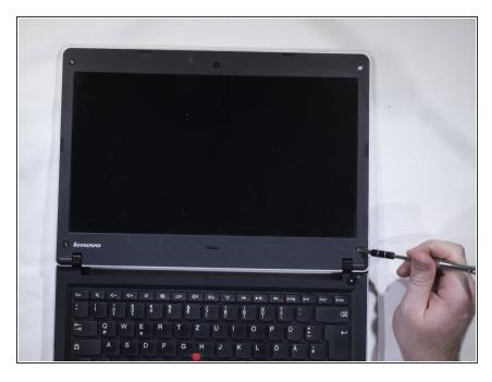
Under each rubber tab is a 4mm long M2 screw. Remove these screws.
