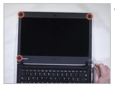
Remove the 4 rubber tabs on the corners of the screen. This can be easily done by twisting them off with the tweezers. The tabs have adhesive on the backs so they can be re-applied later.
