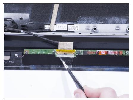
Place the screen face down on the keyboard. The only connection the screen has to the laptop is now its connection cable. There is a piece of tape covering the screen's connection cable. Using the tweezers, remove this tape.
