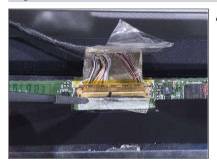
• Underneath the tape there is an exposed connection. The connection cable that plugs into the screen has a securing wire lock that locks the connection in place. The locking wire has a piece of tape that secures it in place to the back of the screen. With the tweezers, carefully peel off this tape.
