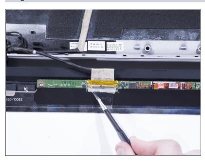
Place the screen face down on the keyboard. The only connection the screen has to the laptop is now its connection cable. There is a piece of tape covering the screen's connection cable. Using the tweezers, remove this tape.
