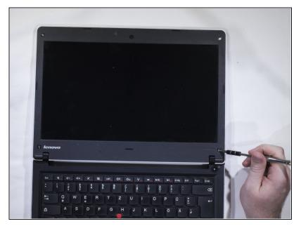
Under each rubber tab is a 4mm long M2 screw. Remove these screws.
