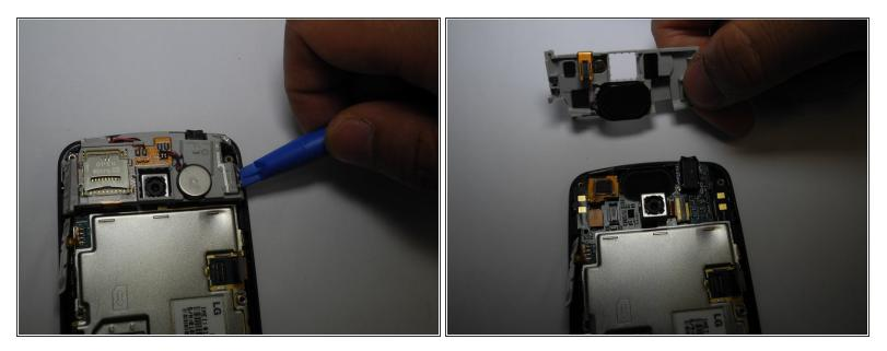
• Remove SD card mount. Insert a plastic opening tool on the right side to pop off.
