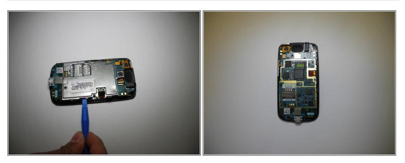
• There are 4 retaining points to insert a plastic opening tool into and pop off panel.
