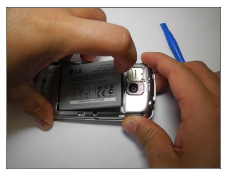
Remove the battery. There's an indentation to the left of the camera lens to pull up on the battery with your finger.
