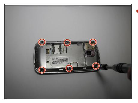
Use a J0 screwdriver to remove the six 4.5 mm screws.
