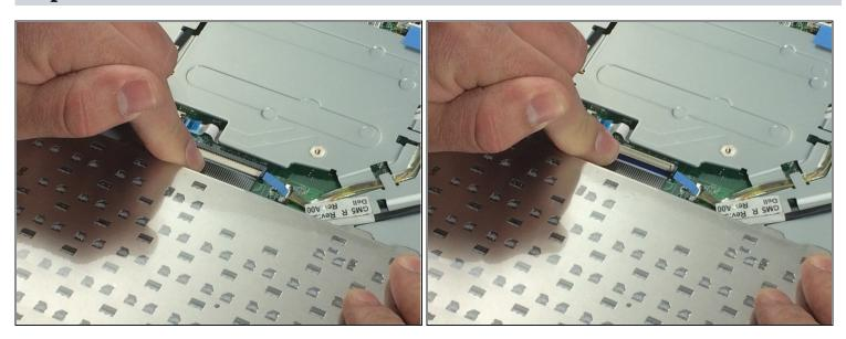
• Remove the ribbon cable as shown
