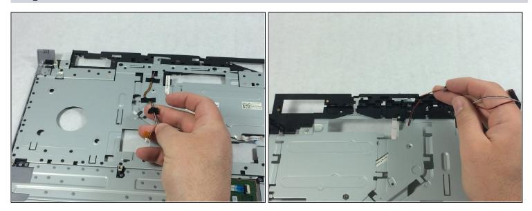
• Peel speaker cables off of the bottom of the palmrest, and route the cable through it such that the speakers are free
