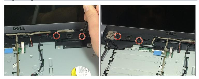
• Remove all four 4mm ph1 screws holding in the speakers
