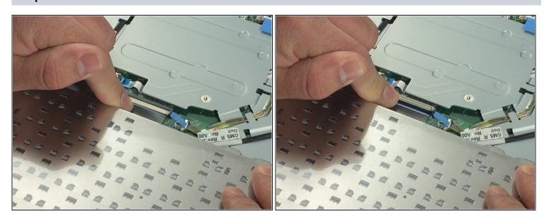
Remove the ribbon cable as shown
