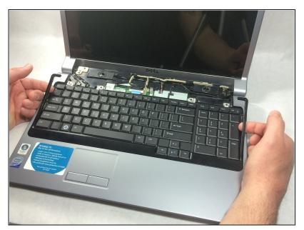
Starting at the top where you just removed the black panel, pry the black bezel away from the outside of the keyboard
