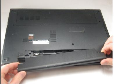
Slide latches outward simultaneously pulling battery out of the laptop.
